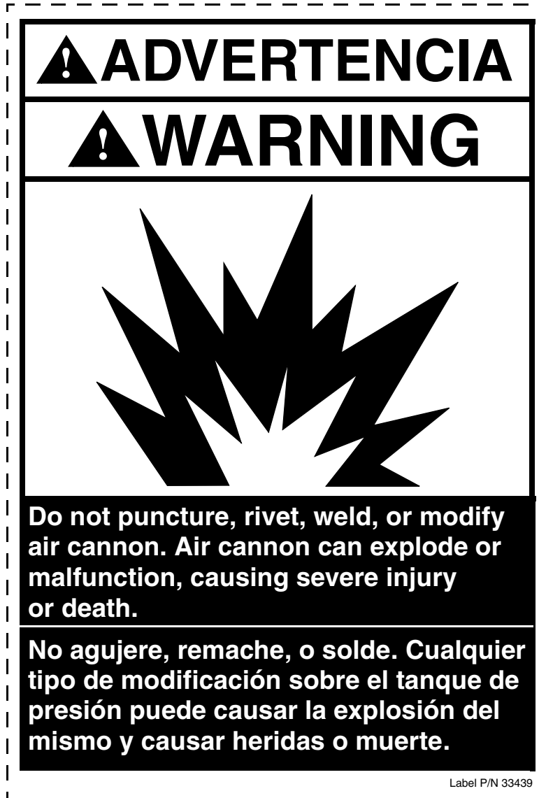
Figure 21. Air Cannon Warning Label, P/N 33439
